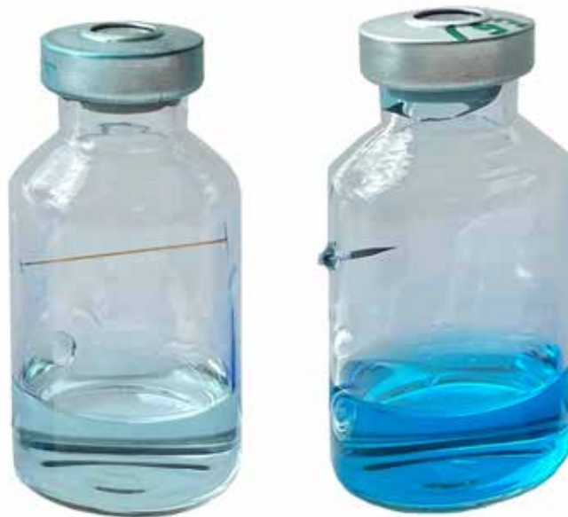
Figure 7.1: Vial with capillary (left) and with micropipette (right) after blue dye test
