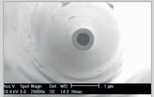
Glass orifice – scanning electron microscope tip image, diameter: 0.4 micrometer
